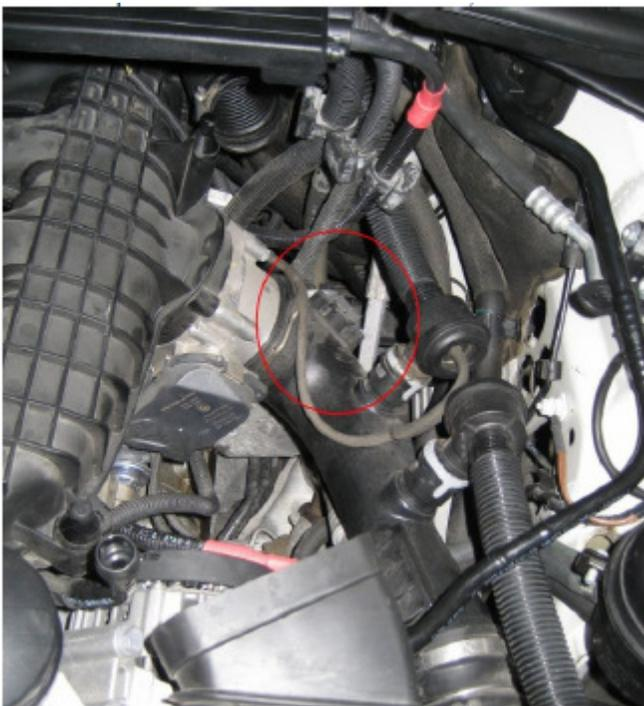
4. Once located, use the flat side of a USB cable to unclip the connector leading to the TMAP sensor. Push the USB cable up until it stays in place on its own, and tug the wire bundle/connector out. Alternatively you may use a penny or screwdriver to lift the clip. If the clip is lifted too far it can break so be gentle. In the event of the clip breaking plug the JB+ in to the TMAP sensor without the clip. Friction will hold it in place.
