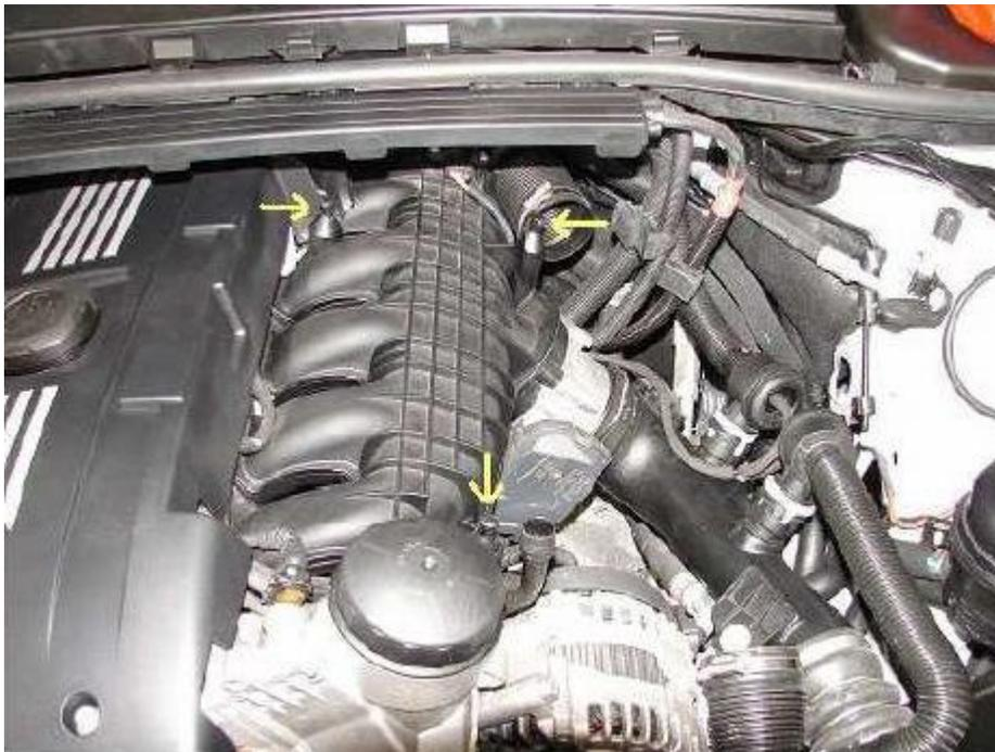
Insert the provided couplers in to each side of the filters and tighten the clamps. The clamps should be snug but take care not to over tighten as you can damage the filter base.
