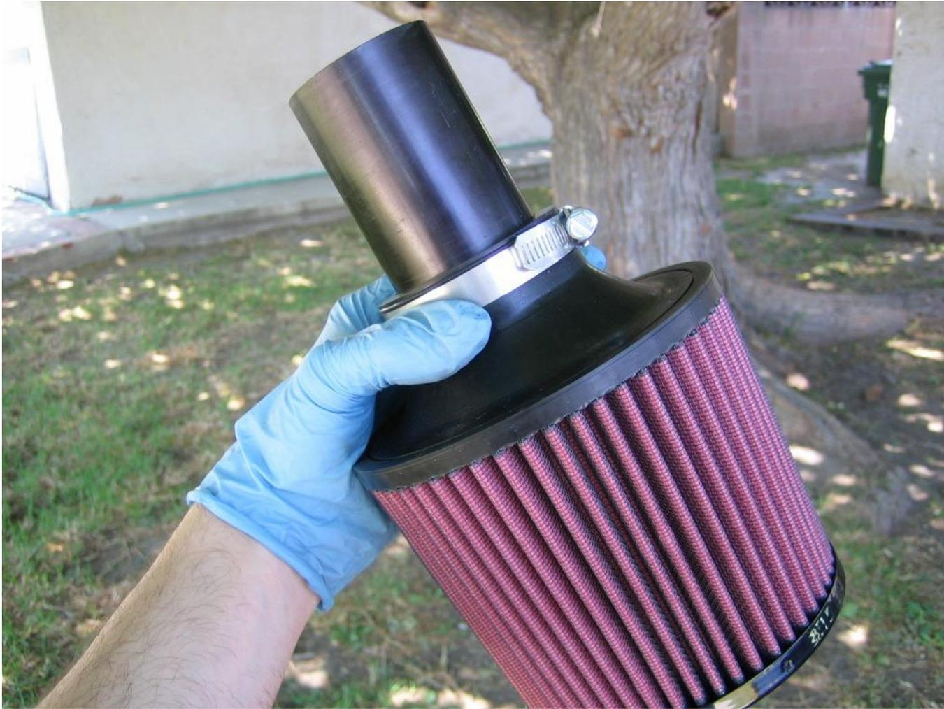
Insert the filter closed to the front of the car first. Slide the intake tube as far in to the factory accordion coupler as it will go, approx 1-2 inches. Tighten clamp.
