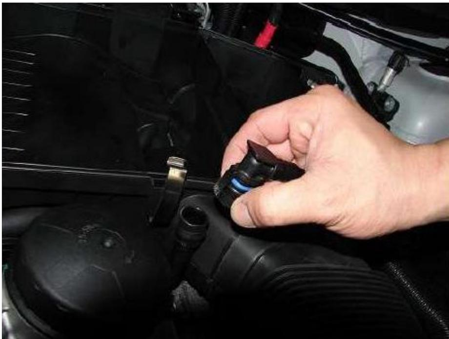
Detach harness by sliding rubber grommets up off air box. If needed use a small screwdriver to help break their seal and pry them up.
