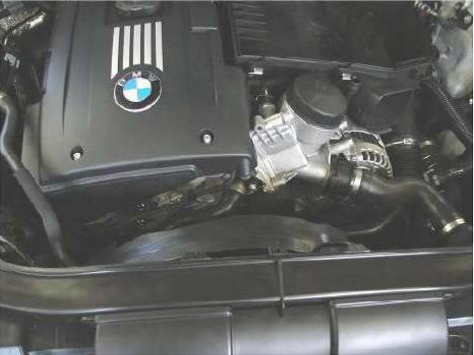
Loosen hose clamps holding inlet tubes to airbox. Many find it easier to pull the battery rail forward, or to remove the cowl entirely. For more detail on these optional steps refer to the JB4 install guide. A 1/4 socket drive (instead of a screwdriver) on the OEM clamps can also make the process easier.
