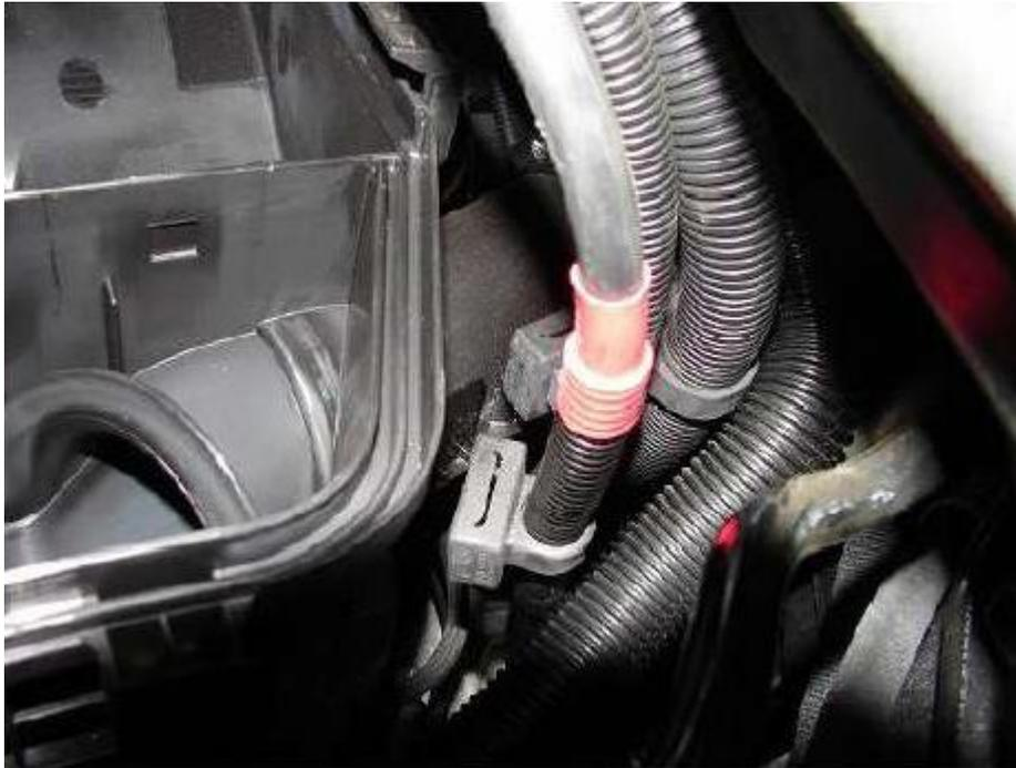
Remove T20 torx screws in the front of the factory cold air scoop.
