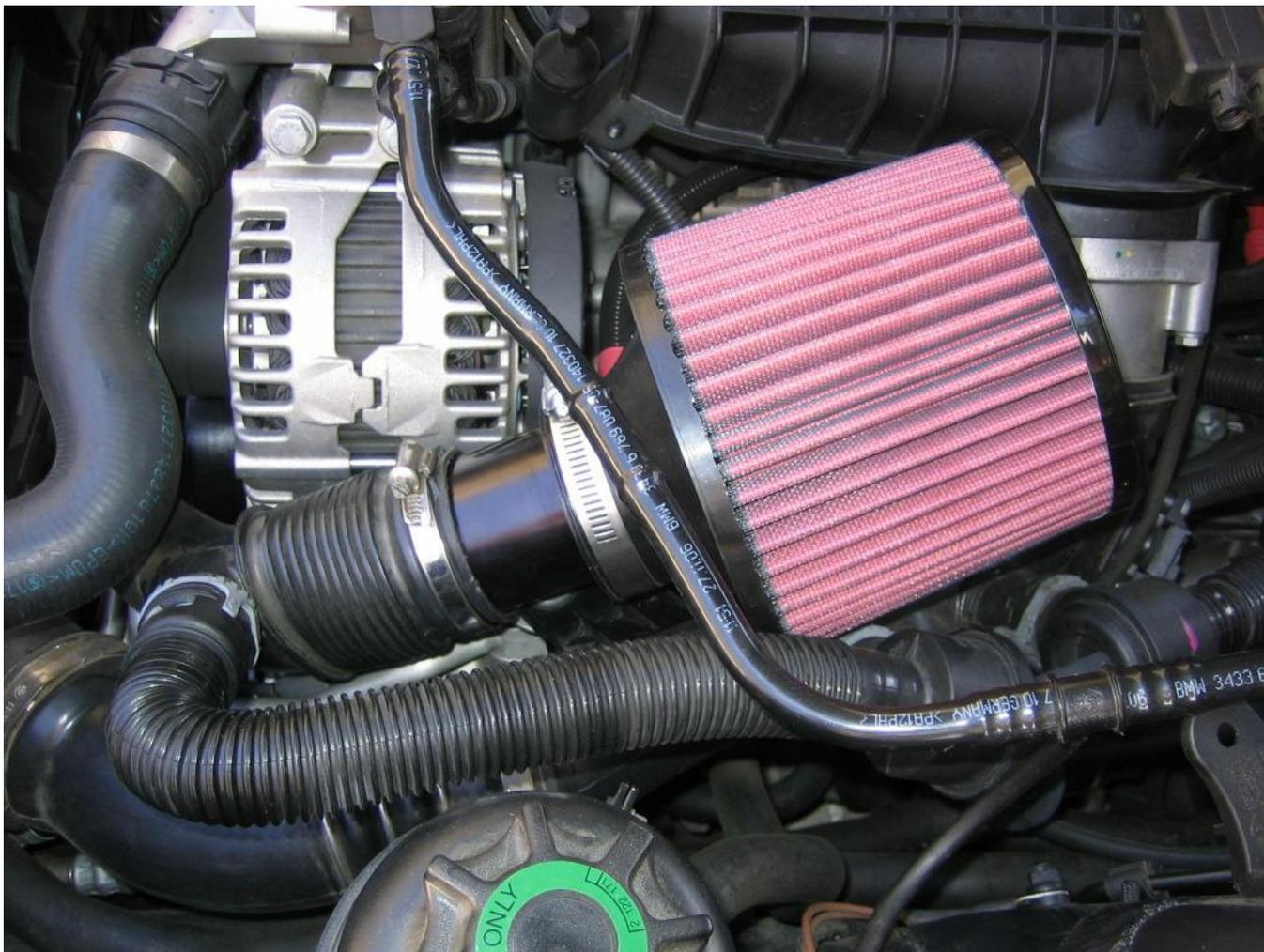
Next position the rear filter. This is the trickiest part of the install process as room is limited and the filter will rub against the front filter and battery cables while being inserted. Stick with it and you'll get it! Having a friend hold the battery cables and front filter out of the way can help. Once inserted tighten clamp.
